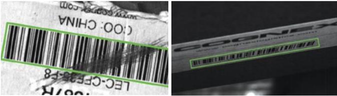
**1DMax™ with Hotbars®** is optimized for omnidirectional 1D barcode reading and decodes low-resolution codes up to 10X the speed of a conventional barcode reader.
