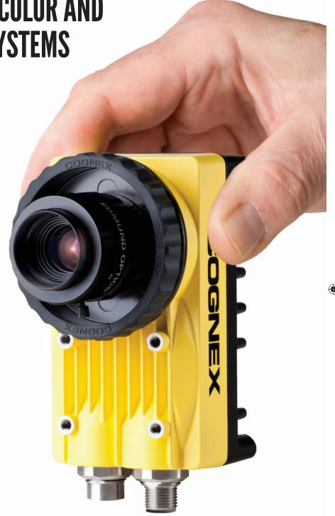
The speed of the 5 megapixel In-Sight 5705 and 5705C systems significantly expands the range of applications that can be solved with a stand-alone vision system.
