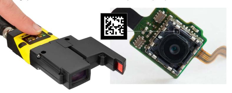
In today's innovative electronics and medical device industries, parts and components are increasingly getting smaller. With little surface on which to mark 2-D codes for identification and tracking purposes, the size of direct part mark (DPM) code cells often end up being 1 mil (25 µm) in size or less.
