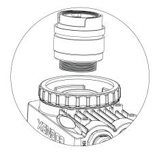
3. If using a lens cover, remove the thread guard and attach the lens to the vision system.
