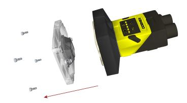
3. Using a screwdriver, loosen the two screws on the LED ring light.
