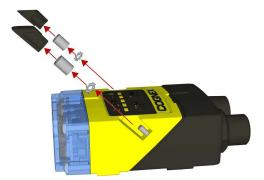
3. Detach the main module and the I/O connector module by firmly pulling them apart.
