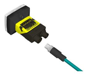
2. Connect the Ethernet cable RJ-45 connector to a switch/router or PC, as applicable. For PoE models, connect the Ethernet cable to a PoE switch port or other PoE sources.
