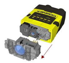
4. Attach a new illumination module. Make sure to attach the illumination module with the correct orientation.
